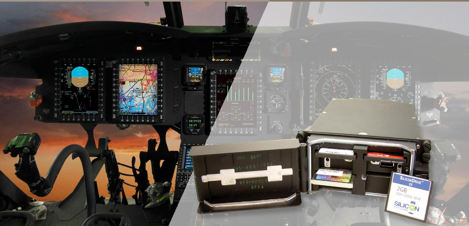
Highly reliable data transfer device, mass storage unit, map database server, video recorder in one small form factor package.
